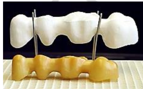
Fig. 36. Volume shrinkage of the restoration after the sintering is compensated by an accurate increase of the milled detail volume
