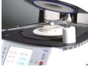
Aluminum oxide plunger is placed above the ingot
