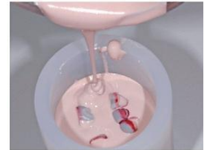
Installing a silicone ring and investing with refractory mass
