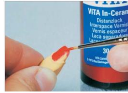
Application of separating varnish onto gypsum stamps (the layer is around 45 µm thickness)
