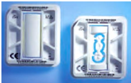
Fig. 35. Ceramic blocks for “soft” milling of ceramic on a base of zirconium dioxide before and after milling
