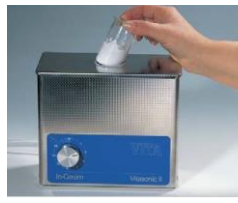
Mixing slip components in ultrasonic device VITASONIC
