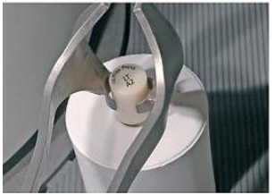
Ceramic ingot is placed into a heated casting box
