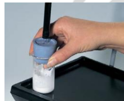
Pumping the air out of the slip with vacuum device
