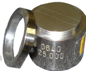
Fig. 2. A test block and a ring form for the assessment of the impression material reproduction of the surface relief, its compatibility with plaster and linear size changes
