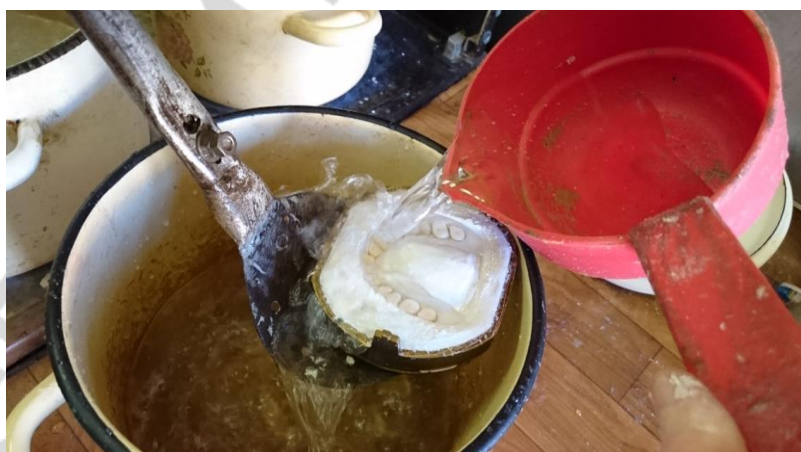
Fig. 58. Removal of wax residues from the cuvette by a hot water jet
