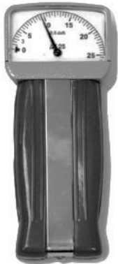
Fig. 4.1. Manual dynamometer (at laboratory room № 131)
