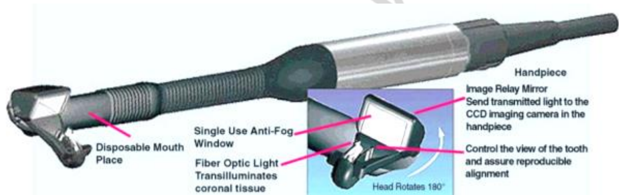
Figure 4. The proximal or occlusal mouthpiece is placed over the tooth in question, allowing light to be shined from one surface, through the tooth, and captured on the opposite side using a CCD camera in the DIFOTI handpiece
