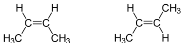
Figure 14. Structural formulas of 2- cis -butene and 2- trans -butene
