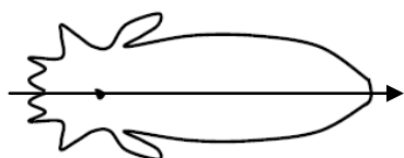
Fig. 3.4. Scattering diagram by particles with size r > \lambda
