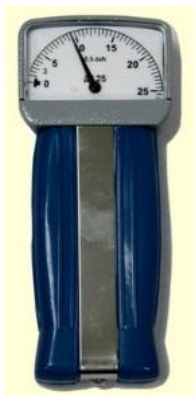
Fig. 4.1. Hand dynamometer (location laboratory room № 131)
