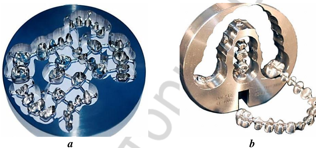
Fig. 16. Frameworks of metal dentures from Co-Cr alloy (a) and Ti-Al-V alloy (b) made by milling with the use of CAD/CAM technology
