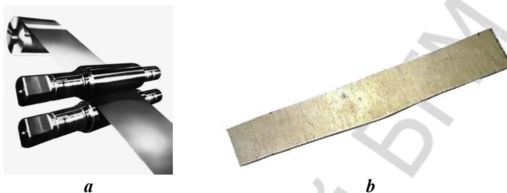
Fig. 2. Two rolling cylinders of a rolling device press a plate ( a ) to produce tape strips of flat profile with 0.3 mm thickness ( b )
