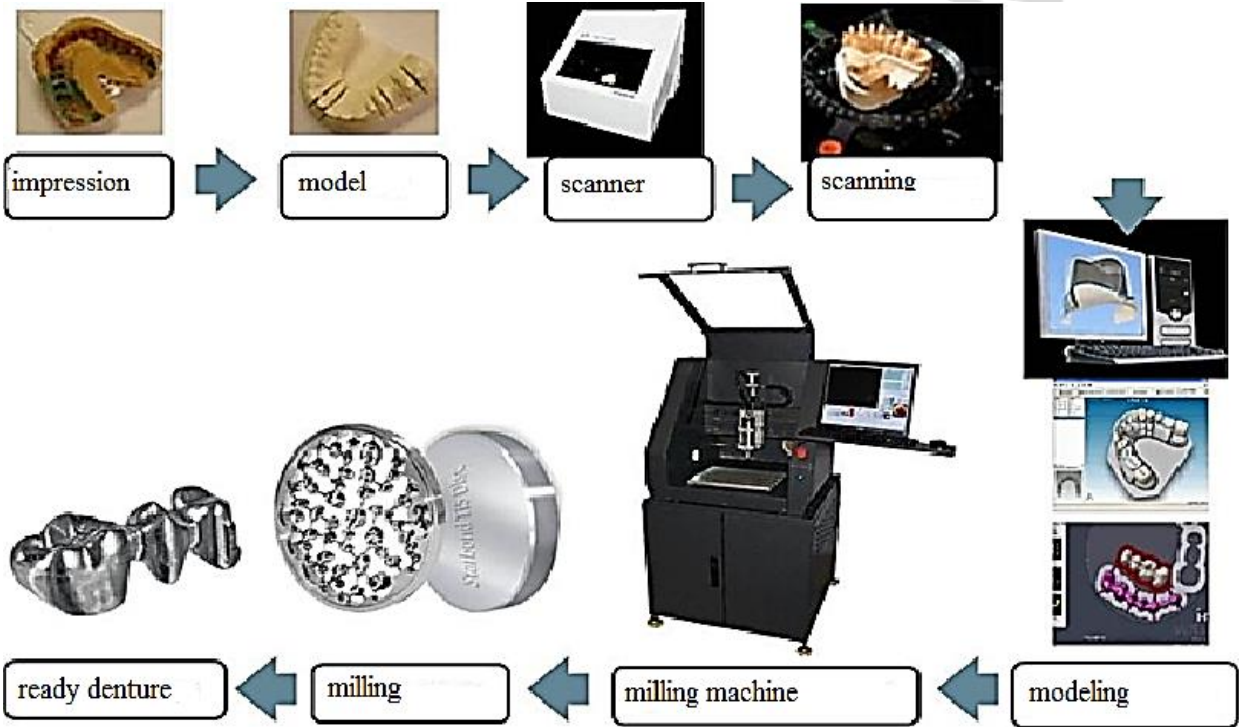
Fig. 15. Sequence of CAD/CAM technology
