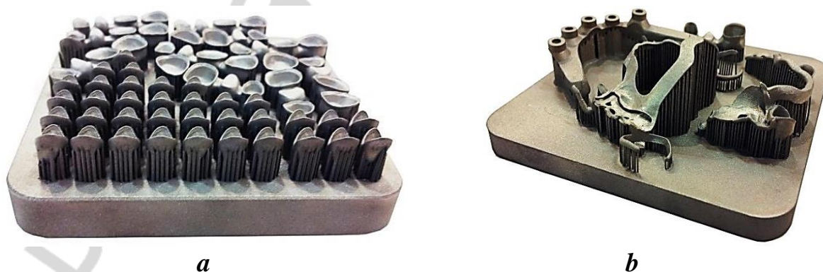
Fig. 18. Metal crowns (a) and metal framework (b) of the cast removable denture made by SLS technology
