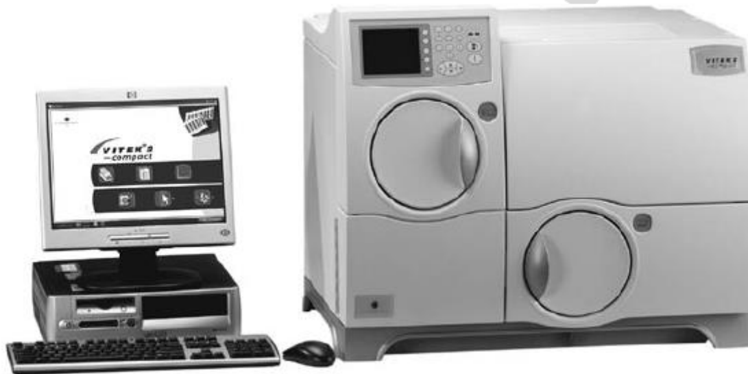
Figure 9.2. Vitek 60 (bioMerieux, France) automated system for identification and susceptibility testing to antimicrobials of microorganisms
