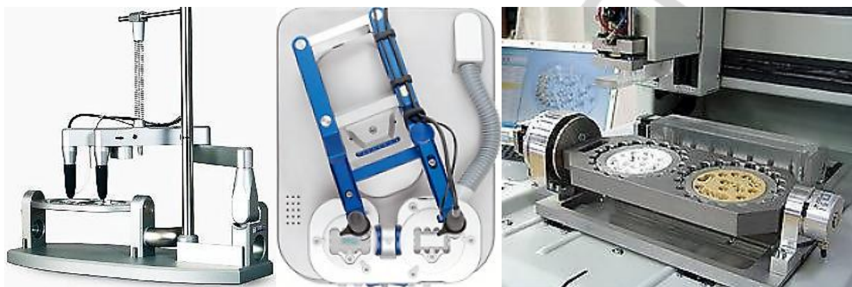
Fig. 38. Milling machine (pantograph) for PSZ frameworks fabrication by copy-milling method
