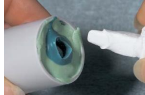
Recovering the model from the mold
