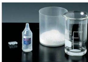
Dozing of slip mass components
