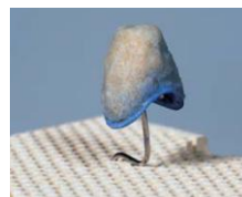
Glass infiltration firing in VITA INCERAMAT furnace
