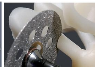
Sprues are cut with a diamond disc
