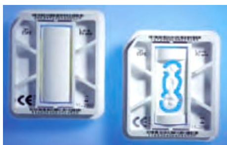
Fig. 35. Ceramic blocks for “soft” milling of ceramic on the base of zirconium dioxide before and after milling
