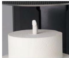
The 1 st sintering of the framework in VITA INCERAMAT furnace
