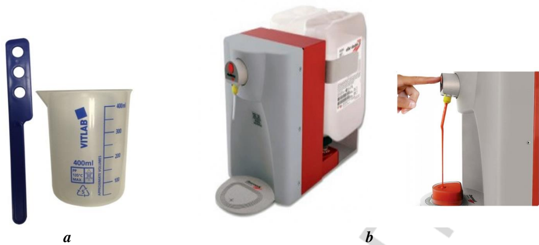
Fig. 4. Container and spatula for manual mixing of vinylpolysiloxane materials (a) and device for automatic mixing of components of vinylpolysiloxane materials for duplication (b)
