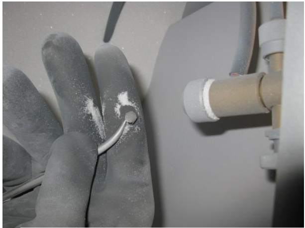
Fig. 45. Sandblasting of a cast cap
