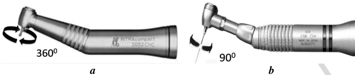
Figure 14. Types of angular micromotor handpieces: a — full-rotation; b — reciprocal
