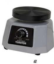
Fig. 6. Plaster Vibration Machine ( a ) and pouring of impression on flat-top working surface of vibrator ( b )
