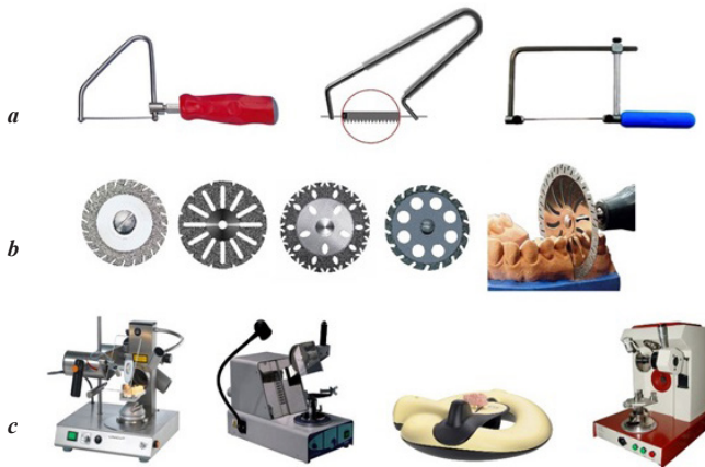
Fig. 16. Tools and equipment used for sawing casts and dies: saw frame with a thin blade ( a ), separating diamond discs ( b ) and special devices for sawing casts and dies ( c )
