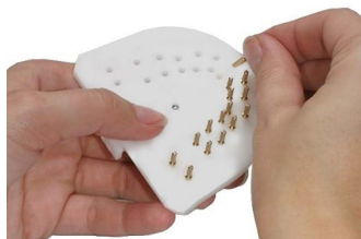
Fig. 28. The insertion of pins into the premanufactured base plate
