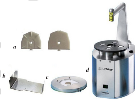
Fig. 25. Tools and equipment necessary for working cast production with separate die system by inserting dowel pins in the premanufactured base plate (the description in the text)
