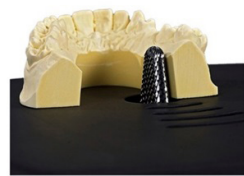
Fig. 19. Plaster milling cutter ( a ) and the process of trimming the cast ( b )
