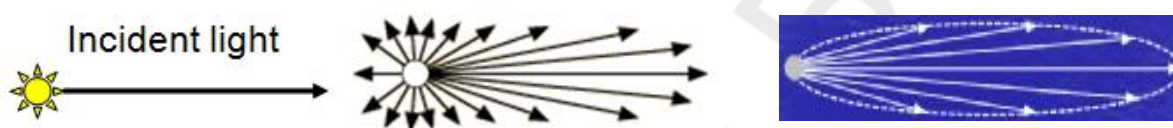
Fig. 20.12. For Tyndal scattering the scattered intensity is more in the forward direction relative to the backward direction
