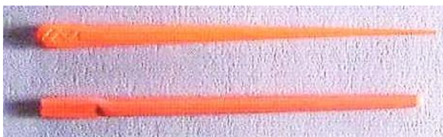
Fig. 3. Nonstandardized (top) and standardized (bottom) cones
